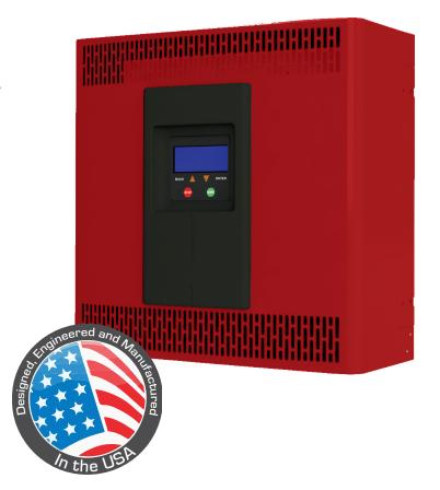
The REVOLUTION Series is an innovative line of ultra-high frequency battery chargers that incorporates cutting edge modular power design that delivers efficiencies greater than 90% throughout the entire charge cycle. As the charge cycle progresses and the output current tapers down, the charger will turn off unneeded modules, allowing the remaining modules to operate at peak efficiency.
