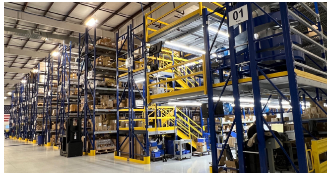
A three-level pick module houses material for manufacturing and assembly. Another on the opposite side of the warehouse houses finished goods.
