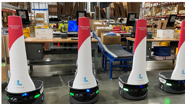
Locus mobile robots deliver orders to induction where they are checked, packed and labeled at new packing stations, then placed on the conveyor for delivery to shipping.
