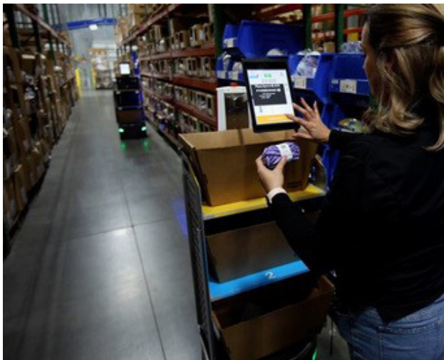
Mobile robots have doubled picking speed to 1,000 orders per day.
