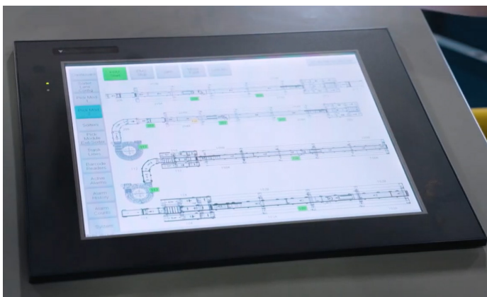
The Wellstar system also includes graphic user interface panels that allow operators to easily monitor throughput rates and troubleshoot system issues.
