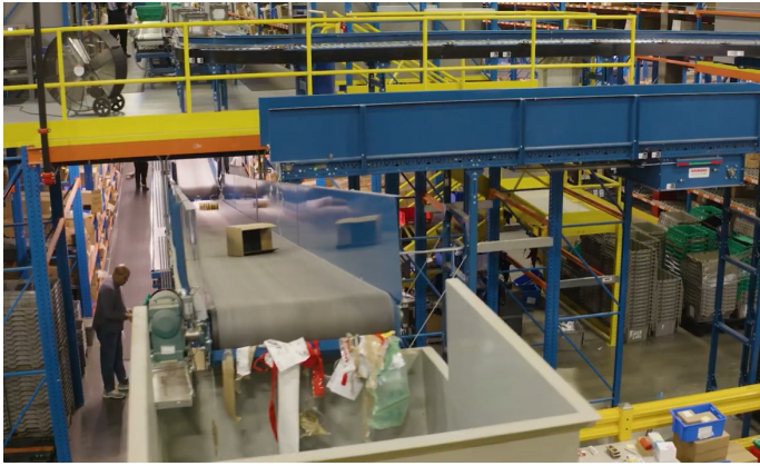
The Wellstar system features an empty corrugated trash conveyor that transports empty boxes to a bailer.
