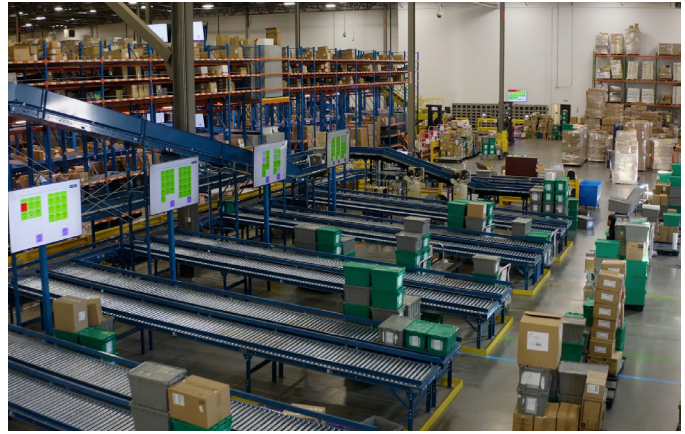
Once the picking process is complete, totes move to a tie-in conveyor that takes them to the shipping sorter.
