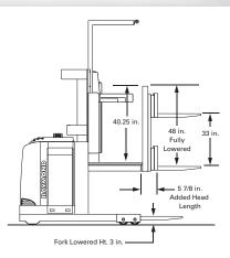
The Mini-Lift Mast is equipped with a pair of forks that allow the operator to lift and lower a pallet, keeping the pallet at waist height for easier pick handling.
