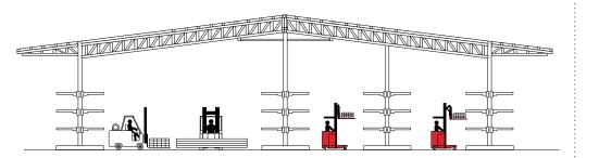
Conventional Storage: Using standard counterbalanced lift trucks, aisles must be wide enough to permit right angle maneuvering with long loads. 7310 4-D Reach-Fork truck: Travel sideways down aisles, eliminate right angle turns, and reduce the potential of loads hitting racks, beams and other stock.
